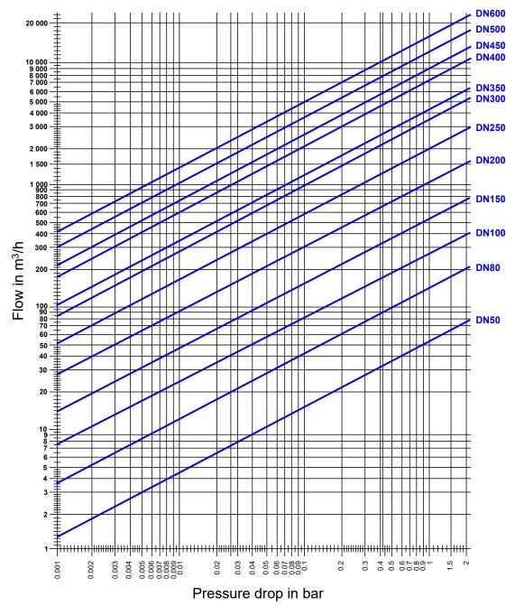
The curves shown on the diagram represent pressure drop related to water at 20° C.
