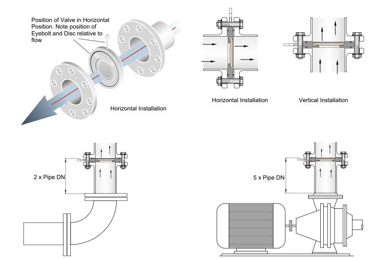
Typical Installation Close to Bends and other Pipeline Components
