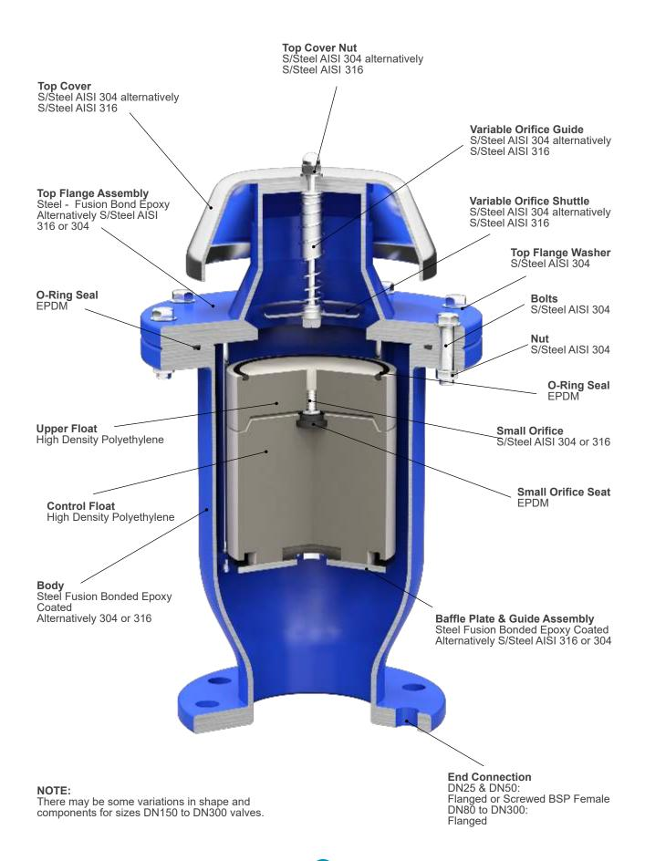
AIRFLO Variable Orifice Air Valves are designed for high performance and low maintenance. The principle of the design is to ensure, through the integrity of the materials of construction, and the performance characteristic of each function that the optimum pipeline performance is achieved with every installed air valve. Some of the features of AIRFLO include:
